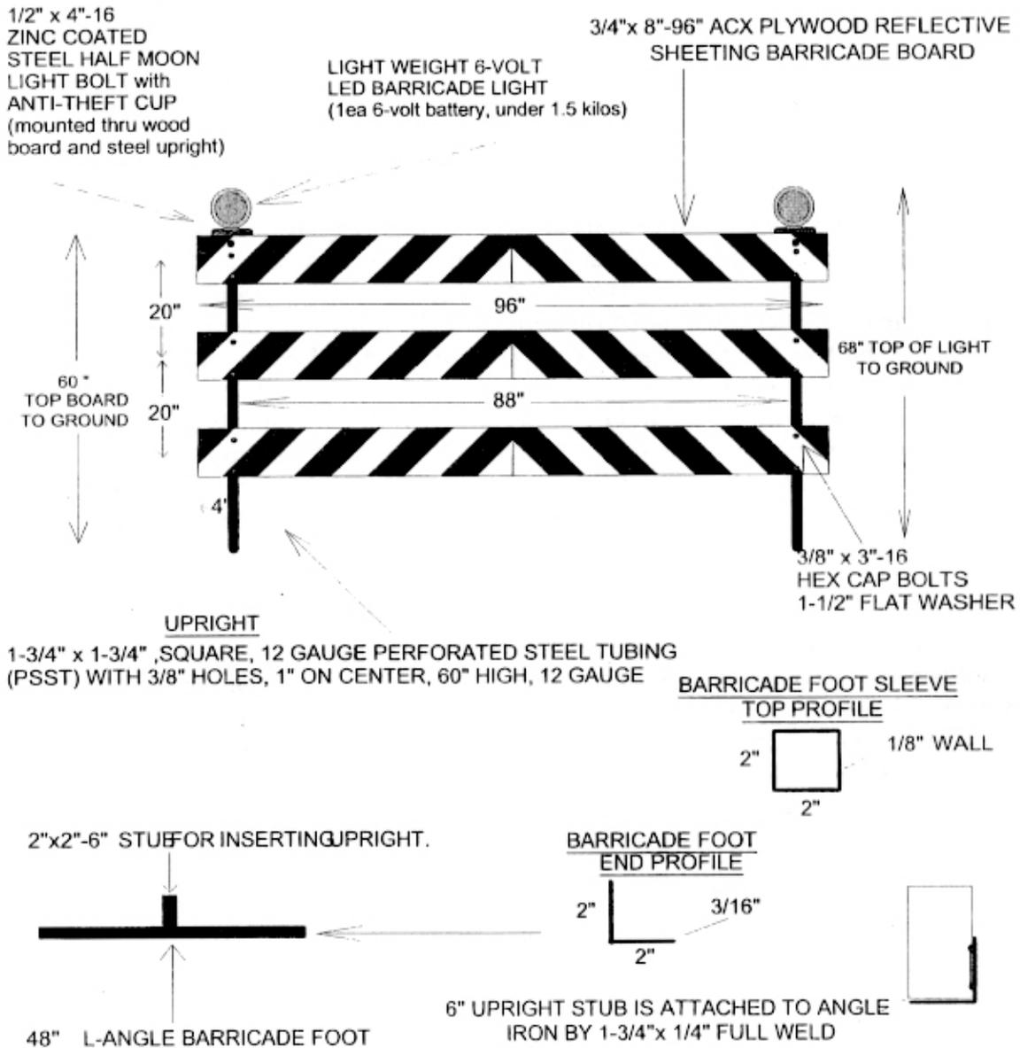
NOTE- BARRICADE IS BALLASTED WITH 8EA, 35LB SANDBAGS FOR HIGH WIND CONDITIONS
